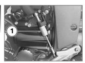
The sensor **1** in the shift linkage detects the shift request and initiates shifting support.
